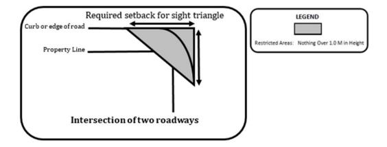
As you can see in the diagram, the sight triangle area shall be measured by connecting straight lines, which are measured from the intersection of the top of the curb adjacent to the two roadways to points established along these lines in accordance with the following distances. Where a road does not have a curb, the edge of the road shall be used to measure the sight triangle.
